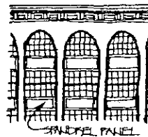
Arcading, with spandrel panels
