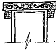
Carved Stone Lintel, with brackets
